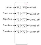
All on: Turn on all 4 zone light. All off: Turn off all 4 zone light. Zone 1-4 on: Short press turn on zone light, long press 1-5s continuous 256 levels increase brightness. Zone 1-4 off: Short press turn off zone light,
