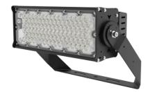
The stadium ESTADIO 300W from the PRIME LED line combines modern technology with high performance. It emits an impressive light stream of 51000 lumens, reaching 170 lm/W. With light colour 5000K provides natural color reproduction, with a CRI of 80. It offers a 90° lighting angle, allowing efficient lighting of large spaces.
